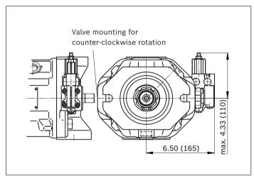
**▼** DRG - Pressure controller, remotely controlled
