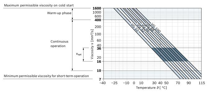
This corresponds, for example on the VG 46, to a temperature range of +4 °C to +85 °C (see selection diagram) 3) If the temperature at extreme operating parameters cannot be adhered to, please contact us.
