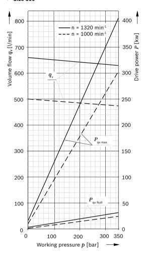
(Operating fluid: Hydraulic fluid ISO VG 46 DIN 51519,  $t = 50 \, ^{\circ}\text{C}$
