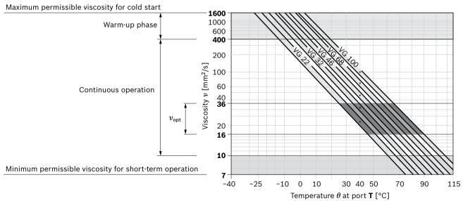
$_{\rm 1)}$  This corresponds, for example on VG 46, to a temperature range of +4 °C to +85 °C (see selection diagram)
